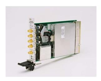
The Rubidium Oscillator provides exceptional longterm stability, while units fitted with the internal oven controlled crystal oscillator also provide clean, low
